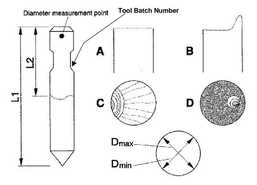
IF CRACKED OR BROKEN, DRAW APPROXIMATE FAILURE LINE IN THE PICTURE OF THE TOOL.
