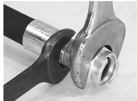
Figure 8-14. Remove Quick Disconnect Coupling Set from Whip Hose.
