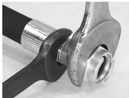
Figure 11-5. Remove Quick Disconnect Coupling Set from Whip Hose.
