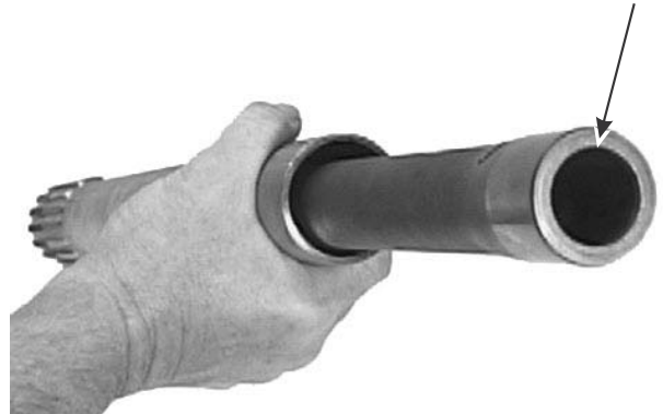
Figure 9-38. Insert Valve into Striker.
