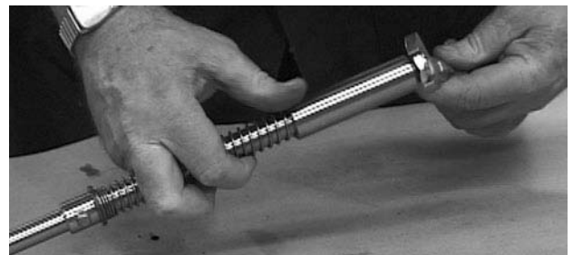
Figure 9-22. Tighten Elastic Stop Nut and Adjust the Valve Play
