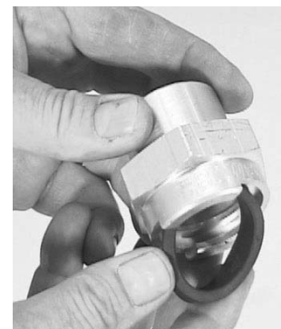
Figure 8-15. Remove Gasket from Socket
