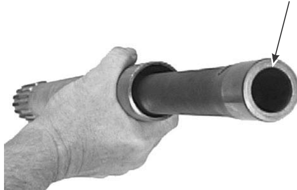
Figure 11-31. Insert Valve into Striker.
