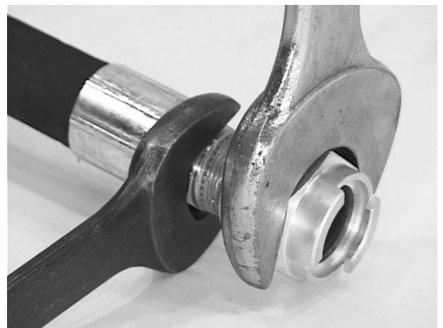
Figure 11-9. Tighten Whip Hose in Q.D. Coupling.
