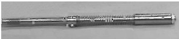
Figure 11-18. Valve Stem Removed from the End Cap.
