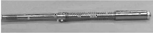
Figure 8-12. Remove the Valve Stem from the End Cap.
