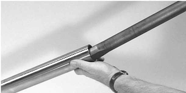
Figure 9-36. Install Striker into Body/Anvil.
