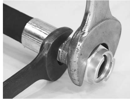
Figure 9-25. Secure Whip Hose to Q.D. Socket.
