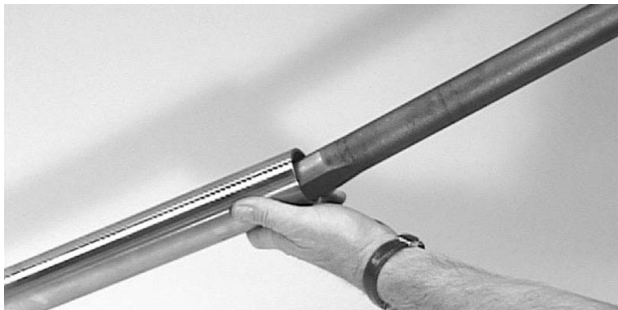
Figure 11-29. Install Striker into Body/Anvil
