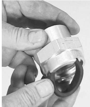
Figure 11-6. Remove Gasket from Socket
