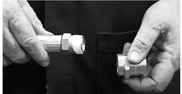
Figure 11-8. Wrap Threads with Teflon Tape.
