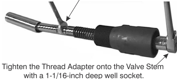
Figure 9-36. Secure the Thread Adapter on the Valve Stem.
