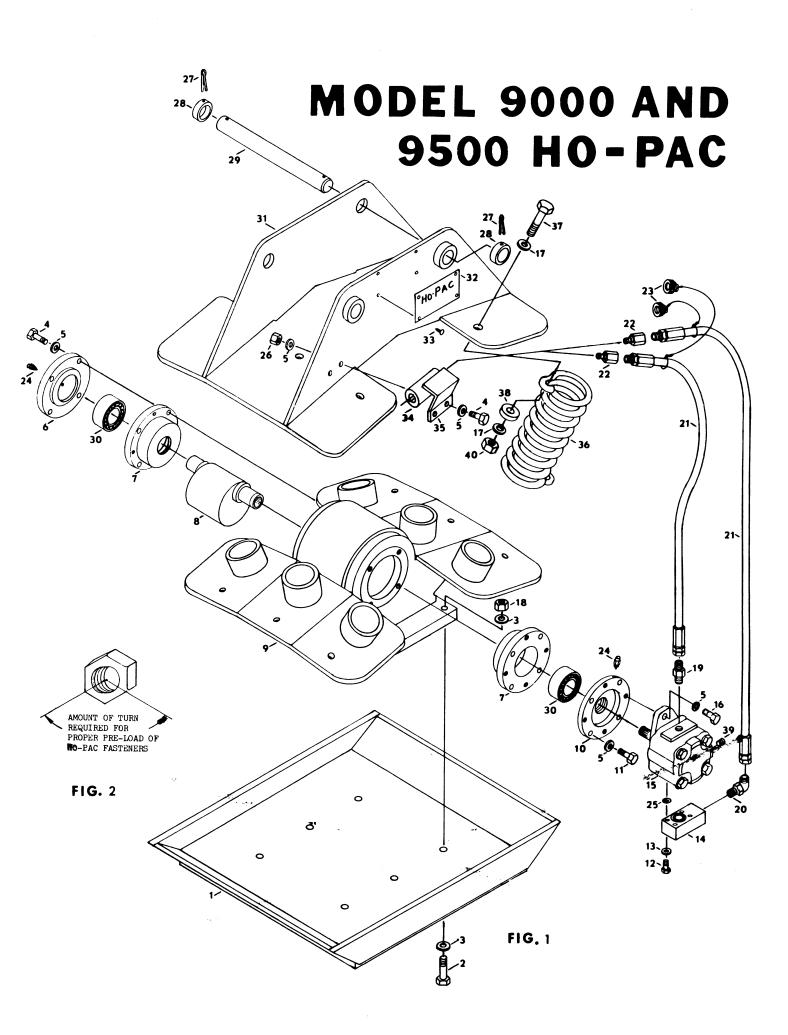
4. INSTALLATION AND OPERATION: Excavators with hydraulic capacities of 33 GPM (at rated pressure) are adequate for simultaneous Ho-Pac and backhoe operation.
