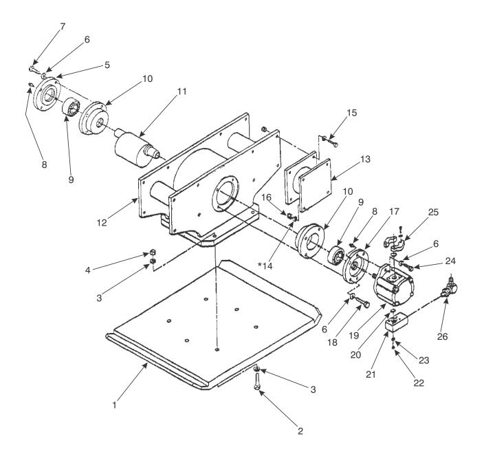
\*NOTE: HARDENED WASHERS, ITEM 14, ARE INSTALLED ON INSIDE SURFACE OF MOUNT, ITEM 13, NOT BETWEEN MOUNT AND FRAME.
