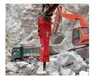
One or more of over 2,500 customized hydraulic kits from Allied provide components for mounting the Model AR 165 and Model AR 175 AR Series hammers on excavators (Model AR 165 on 73,000-90,000 lbs. and Model AR 175 on 88,000-154,000 lbs.).
