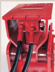
Hoses have been re-positioned
