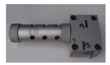
The AutoLube (HR 200 through HR 1200) provides lubrication of the Hy-Ram hydrualic impact hammers with a compact cartridge mounted with a clamp or a bracket that is welded to the housing. It is operated by the hammer's vibration (no hydraulic pressure is required). As a result, there is a more continuous flow of lubricant from the cartridge as it dispenses around the demolition tool and wear bushings.
