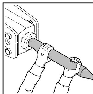
Note: If hammer is still on carrier, it may be easier to stick the tool in the ground and lift the hammer off the tool. Make sure that the tool can not fall.
