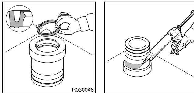
5. Lubricate the contact surfaces of the front head. Leave 50 mm area from the opening of the hole clean from lubricant. Do not allow the silicone compound and the thread grease get mixed.
