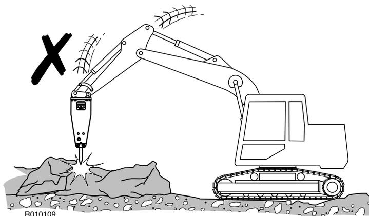
4. Use the excavator boom to press the hammer firmly against the object. Do not pry the hammer with the boom. Do not press too hard or too gently with the boom. The correct force is applied, when the tracks start to lift slightly from the ground.
