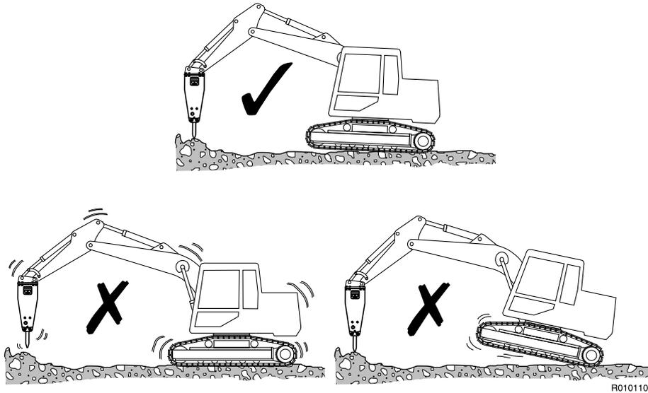
5. Place the tool against the object at a 90 degree angle. Avoid small irregularities on the object which will break easily and cause either idle strokes or an incorrect working angle.
