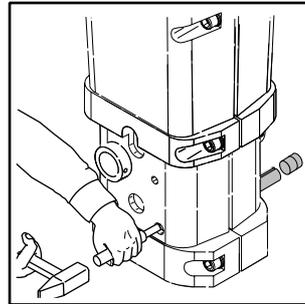
4. Remove lower tool bushing and upper tool bushing.
