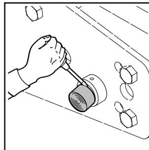
6. Remove tool retaining pins.
