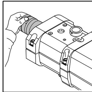
5. Remove seal from lower tool bushing.
