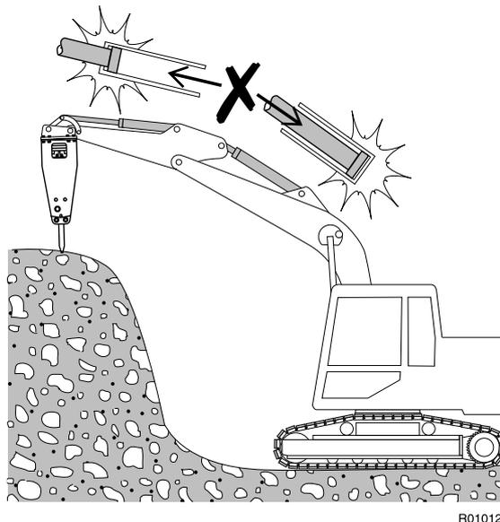
20. Do not use the hammer or hammer tools for lifting. Lifting eyes on the hammer are for storage and maintenance purposes only.
