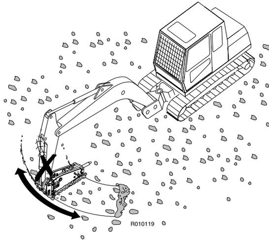
18. When operating the hammer, make sure that it does not make contact with the carrier boom or hydraulic lines.
