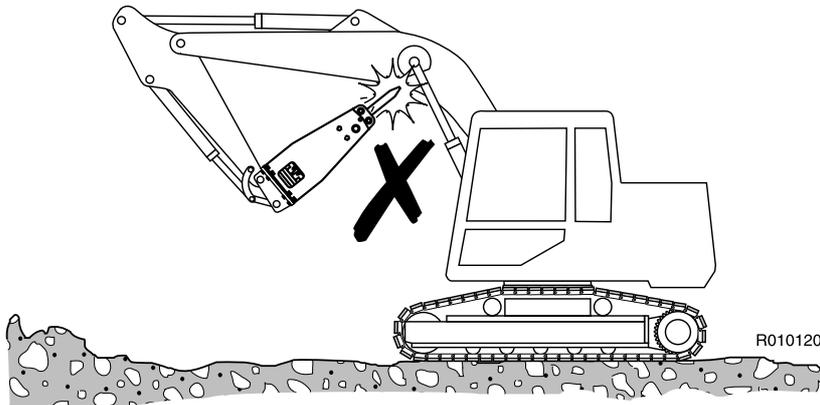
19. Do not operate the hammer with the carrier's boom stick or bucket cylinders at the end of their stroke (either fully extended or retracted). Damage to the carrier may result.
