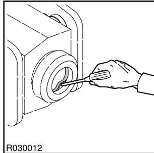
5. Clean and coat tool and retaining pins with grease.
