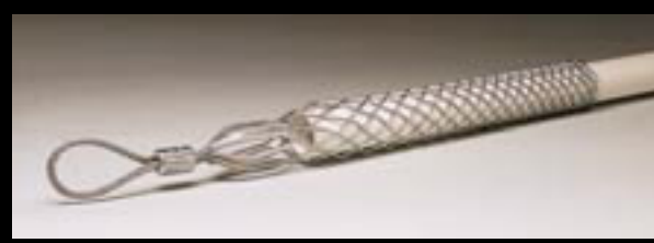
Pulling Grips Simple attachments for the Red-Hog Express that work on a leverage principle by gripping small I.D. pipe and cable and pulling the I.D. pipe and cable in the forward or reverse directions through the tunnel. Available in 7 sizes: 3/4" to 1", 1" to 1 1/4", 1 1/4" to 1 1/2", 1 1/2" to 1 3/4", 1 3/4" to 2", 2" to 2 1/2" and 2 1/2" to 3".
