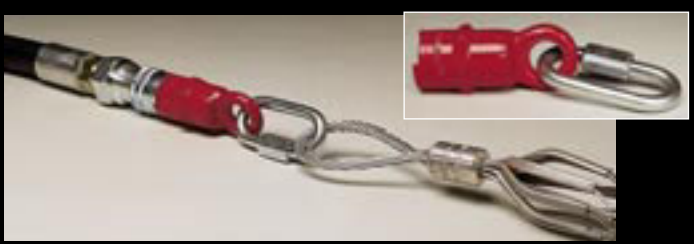
Supply Hose Pulling Adapter Assembly Coupled to the supply hose, the Pulling Adapter Assembly consists of a connector and a threaded chain link. After completion of the tunnel, the supply hose is disconnected from the Red-Hog Express and attached to the Pulling Adapter Assembly which is connected to a Pulling Grip holding a utility service. The utility service is then pulled through the tunnel.
